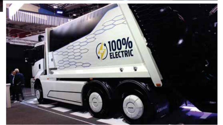
The first all-electric Ford truck is reminiscent of the F-Max long-haul truck series. The three-axle truck is equipped with a refuse collection body and is expected to have a maximum range of 300 kilometers.
