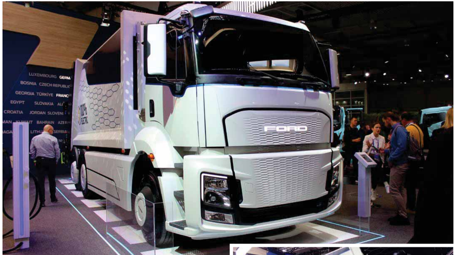
The first all-electric Ford truck is reminiscent of the F-Max long-haul truck series. The three-axle truck is equipped with a refuse collection body and is expected to have a maximum range of 300 kilometers.
