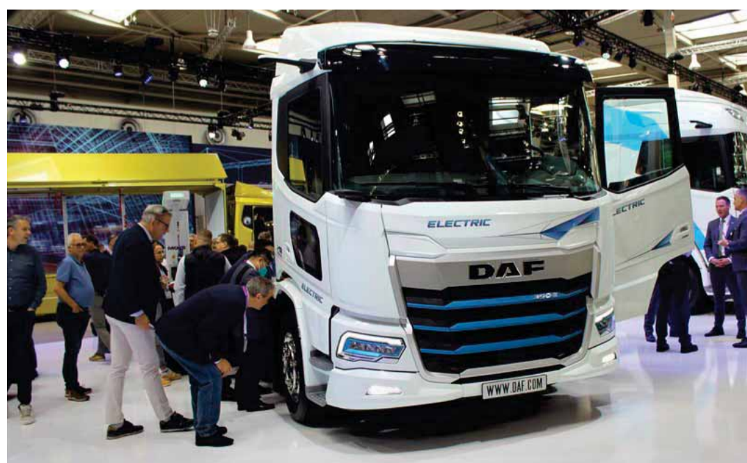
The Electric version of the DAF XD can be recognized by its blue radiator grille slats and headlights with a blue background. In the top version, it is 350 kW and 1,975 Nm strong.
